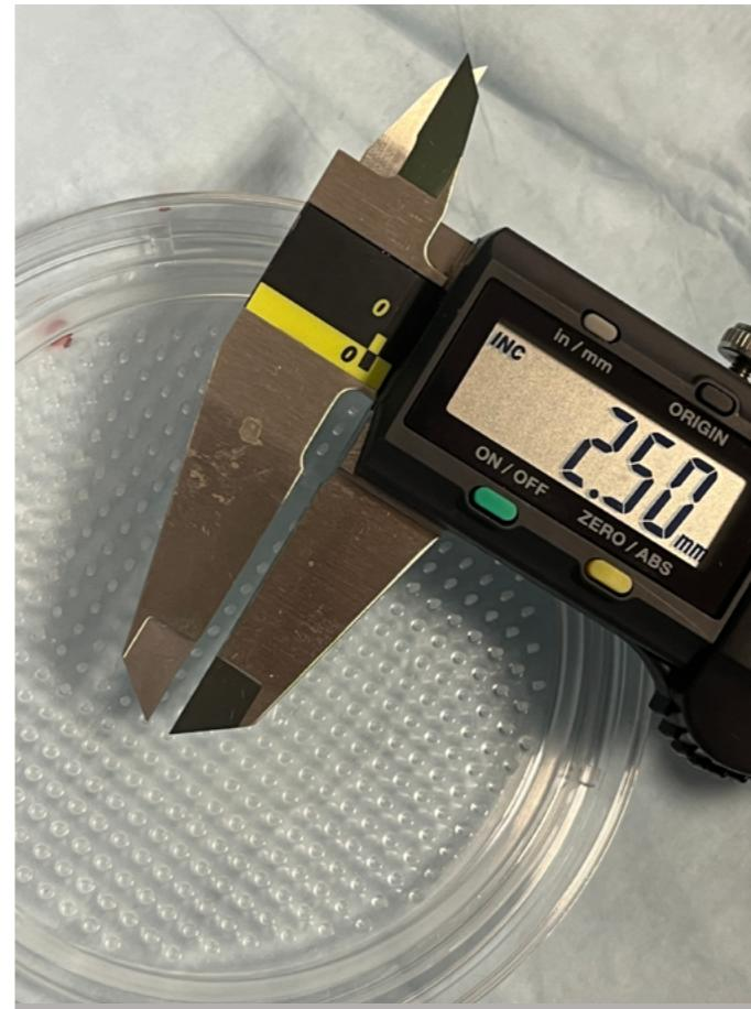
Measuring the dimensions of the PDMS molds prior to the experiment for reproducibility purposes.
