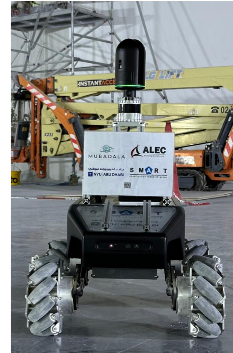
Robotic platform with Leica BLK360 LiDAR being tested in one of ALEC's project in Saadiyat Island.
