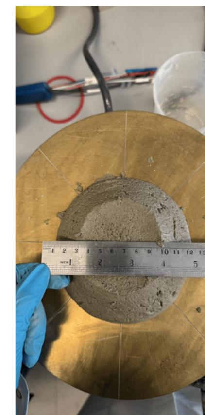
Testing the workability of mortar.
