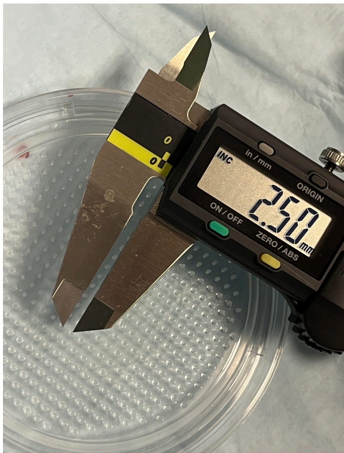
Measuring the dimensions of the PDMS molds prior to the experiment for reproducibility purposes.
