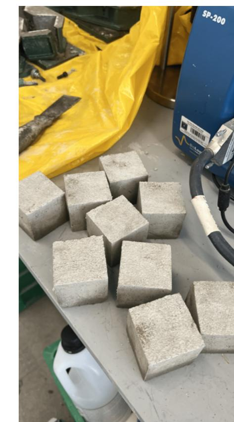
Mortar samples for compressive strengths.
